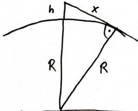
$$\begin{aligned} R^2 + x^2 &= (R+h)^2 \\ &= R^2 + 2Rh + h^2 \\ \Rightarrow x &= \sqrt{2Rh + h^2} \end{aligned}$$
